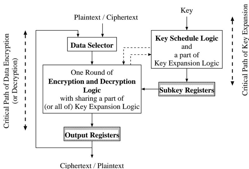
**Figure 2:** Outline of Type 2 (ASIC, FPGA)
